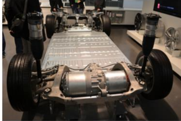
Chassis of Tesla Model S displaying Batteries and Motors
