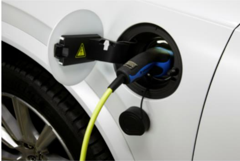
EV Charging Connector
